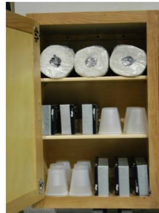
Figure 4. Kitchen cabinet with tissue box ignition source and view inside a loaded cabinet.
