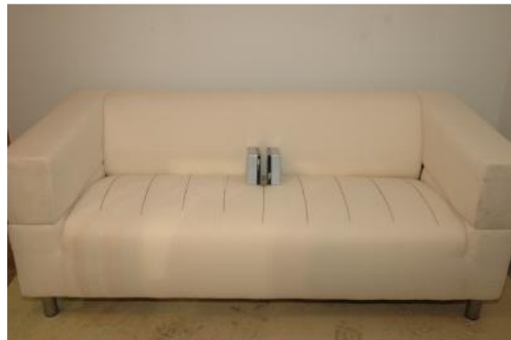
Figure 3. Sofa B used for smoldering fire test SM4 (left) and sofa A with tissue box ignition source used in flaming fire test S1 (right).
