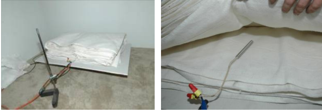
Figure 5. Cotton batting and cartridge heater used for smoldering source.
