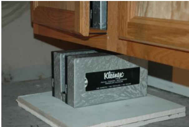
Figure 4. Kitchen cabinet with tissue box ignition source and view inside a loaded cabinet.
