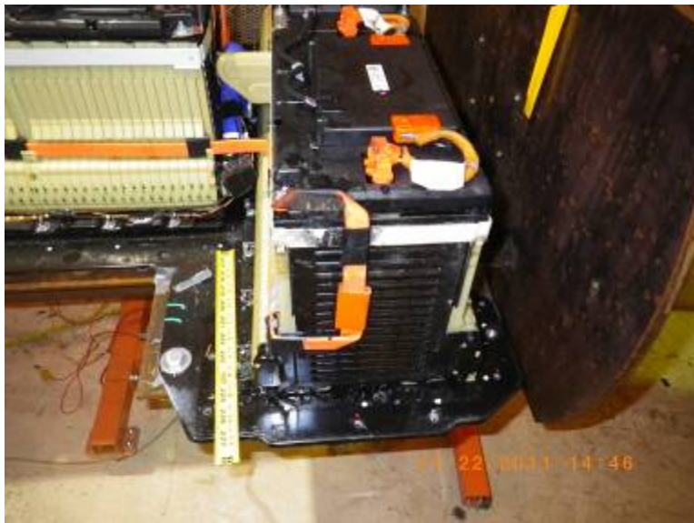
Figure 7.16 – Arcing Damage at the Driver’s Side End of Module 3
