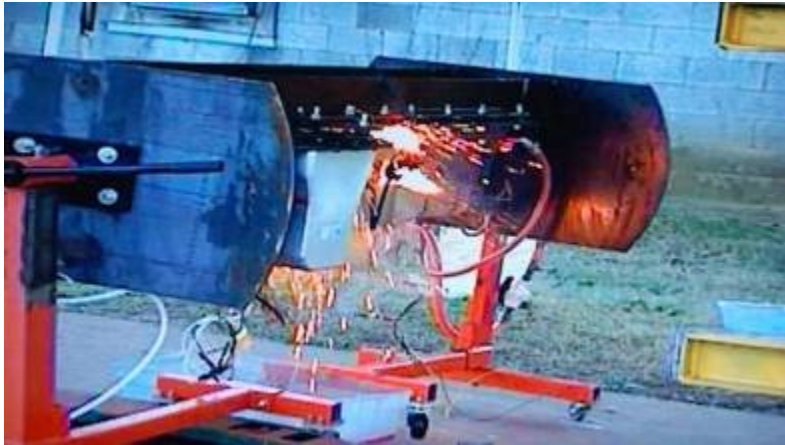
Figure 7.11 – Photograph Showing Flames and Sparks from Test 3 Battery
