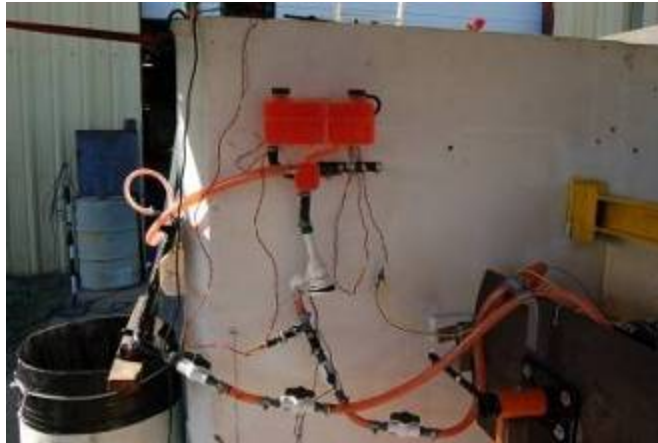
Figure 4.8 Battery Cooling System Test Setup
