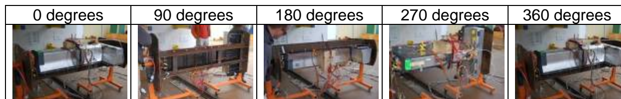
Figure 5.2 Battery Rollover Photographs
