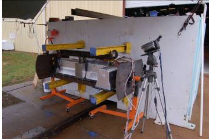
Figure 5.1 Thermocouples & Gas Detection Instrumentation connected to Battery
