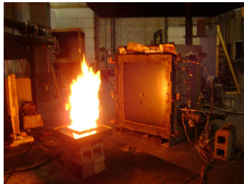
300°C hot surface with n-Heptane pool fire
