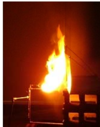
horizontal lube oil spray
