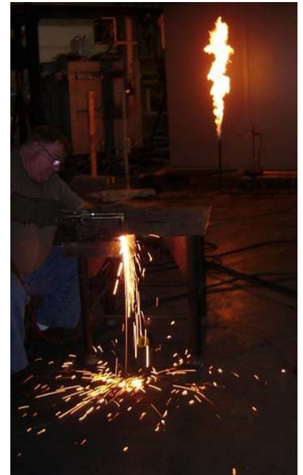
Metal torch cutting
