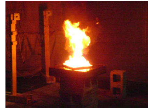
Diesel Pool (48 kW)
