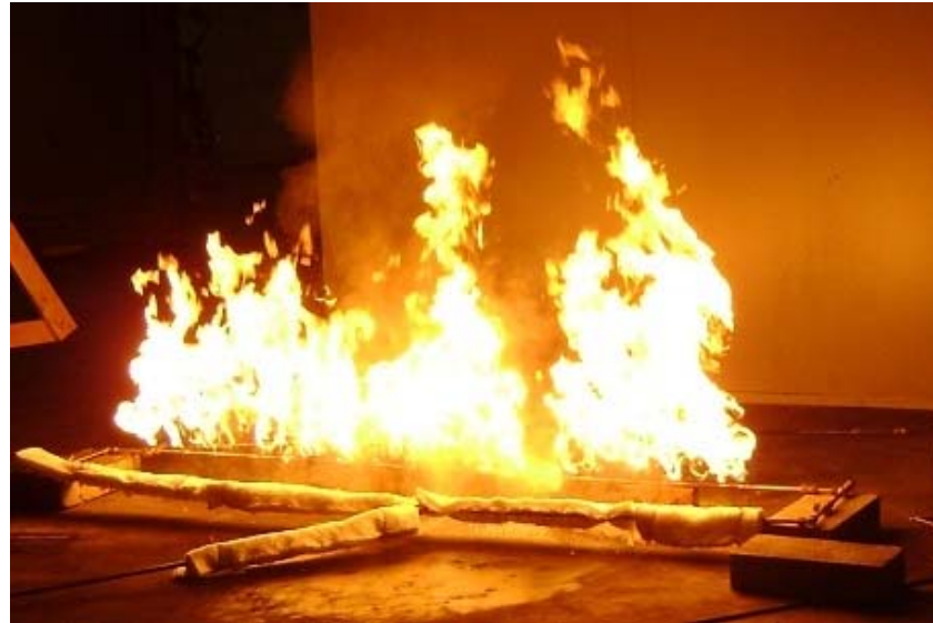
Propane Line Burner (248 kW peak)
