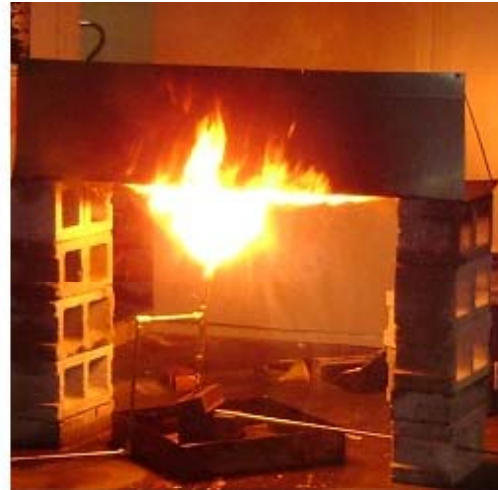
vertical lube oil spray
