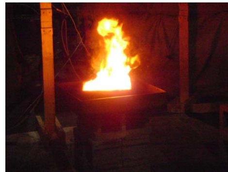
Lube Oil Pool (37 kW)
