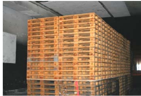
Figure 3. Typical fuel array using 252 softwood Euro-pallets.
