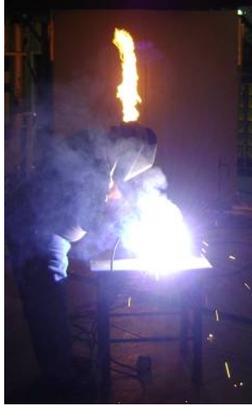
Figure 10. Arc welding nuisance with a vertical natural gas jet flame.
