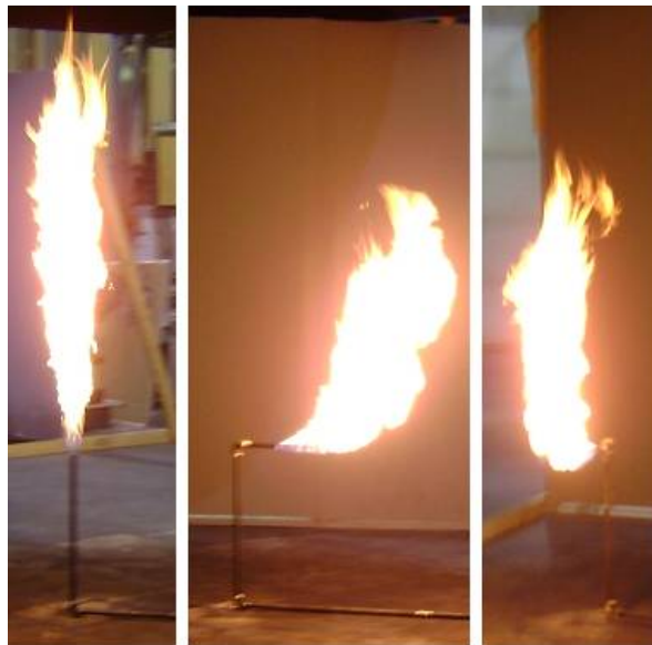
Figure 3. Vertical, perpendicular horizontal, and parallel horizontal natural gas jet fires.
