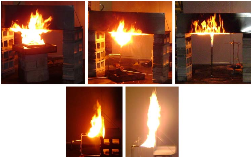
Figure 9. Impinged fires, from top left n-heptane pool, vertical lubricant oil spray, vertical natural gas jet; bottom row, horizontal lubricant oil spray, horizontal natural gas jet.
