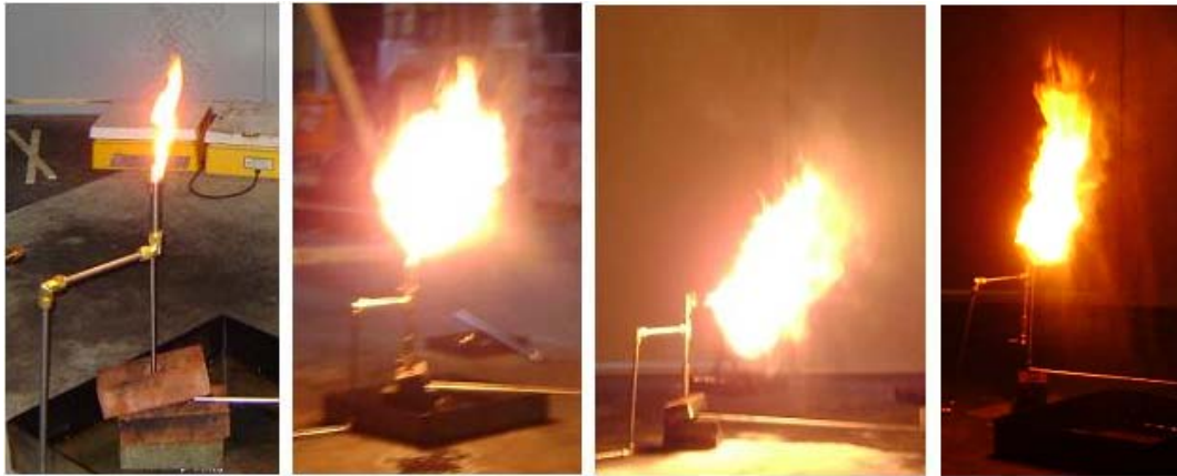
Figure 4. Photos of pilot light and lubricant oil spray fires (vertical spray, perpendicular horizontal, and parallel horizontal spray from left to right).
