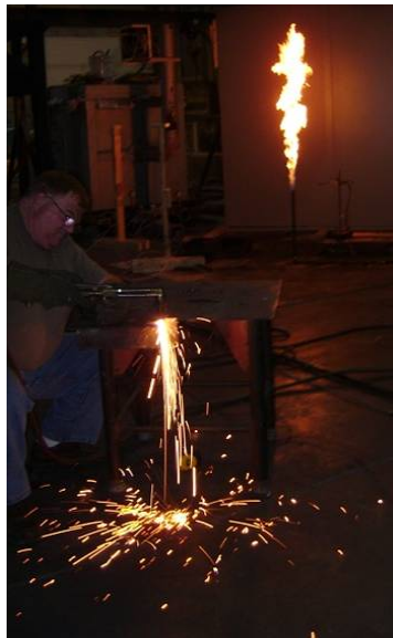
Figure 11. Metal torch cutting nuisance with vertical natural gas jet flame.
