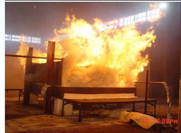
Fire test of x by 3y mock-up with hood in the down position.
