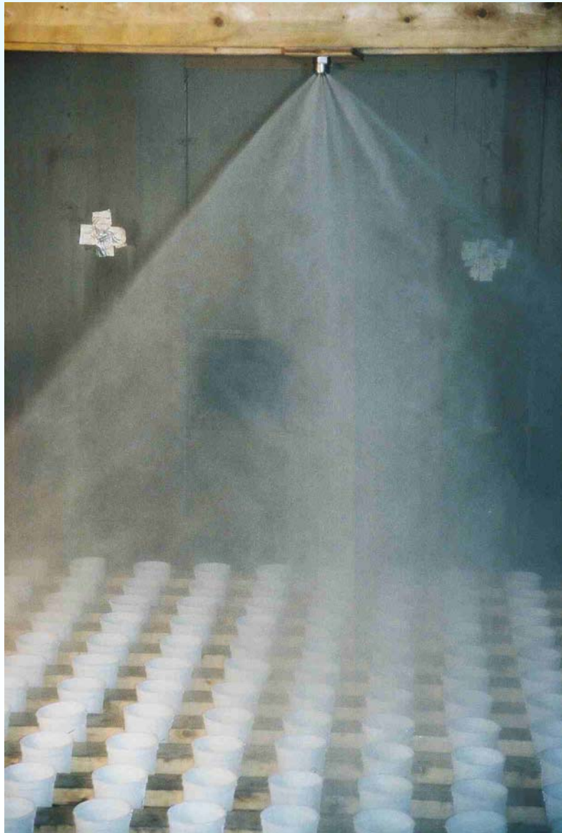
Water mist nozzle spray characterization – flux distributions
